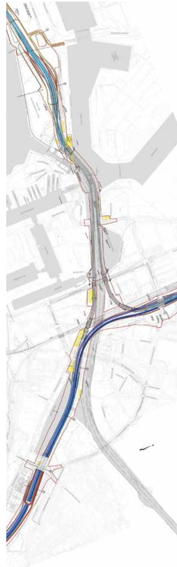
Grondplan cut and cover tunnels. © TV SAM
